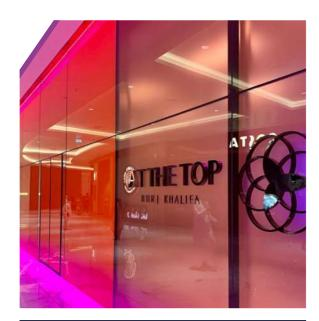
Client: Emaar **Architect:** GSM Façade Consultant: WSP Contractor: Seele Middle East **Product: SPECTRO**VIEW (25mm laminated glass using two panels of 12mm Ultra Clear and bespoke Vanceva® colours)
