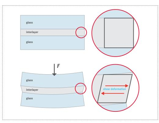
Laminated safety glass with SentryGlas® interlayers react quite differently to PVB interlayers. In tensile tests, the strength of SentryGlas® is considerably higher than PVB. In addition, the stiffness of SentryGlas® is up to 100 times greater than PVB.
