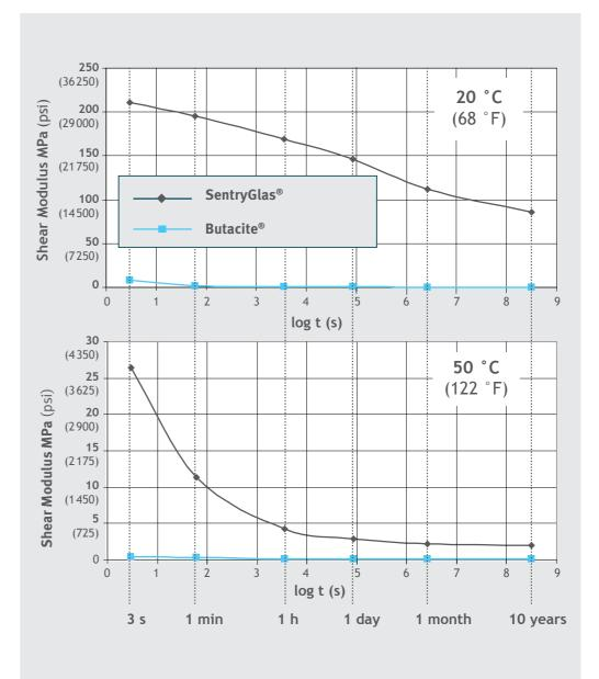
When designing static-loaded laminated glass panels, structural engineers must consider the changes in the mechanical properties and behavior of the interlayer, in particular, the constraints when using PVB rather than SentryGlas® ionoplast.
