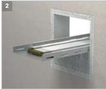
2 Coat cables and cable trays with ROKU® MFC 100 and adjust ROKU® MFP mineral fibre panels on both sides of the wall/ceiling.
