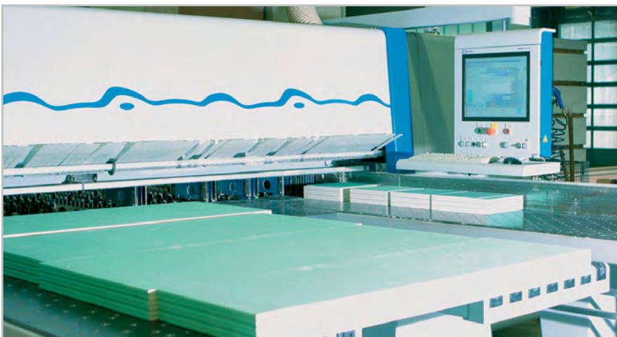
Modern CNC controlled board-separating saw for individual and fully automatic cutting processes with extreme accuracy.
